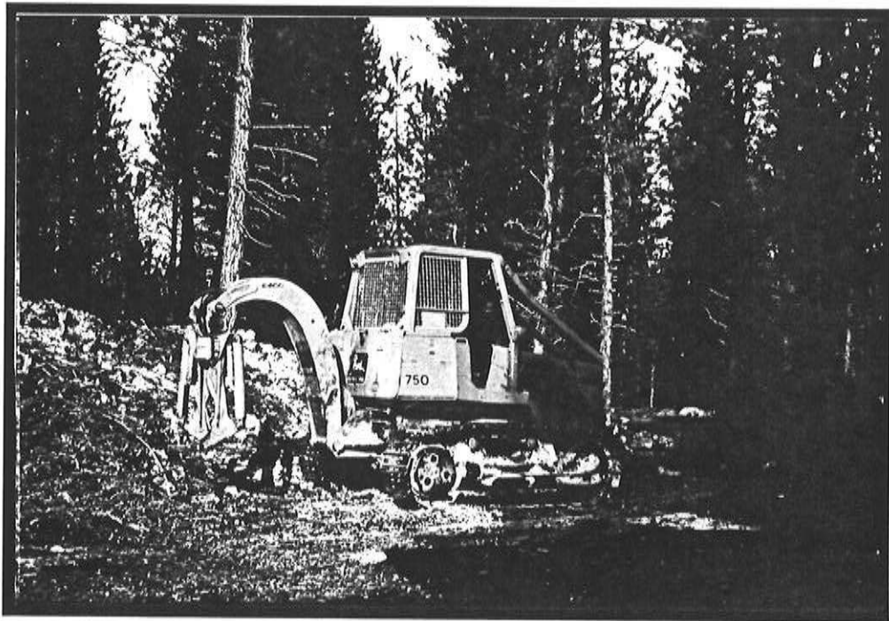
Mechanical precommercial thinning equipment: A Clipper (above) and a Grapple Tractor (below), 1985. (Photos: T. Roberts, Nez Perce Tribal Forestry Office)
