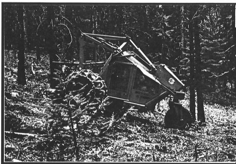
Mechanical precommercial thinning equipment: feller buncher on the Mud Springs Reserve, T.U. 11 as part of the Hog Fuel Operation, 1982-85. (Photo: T. Roberts, Nez Perce Tribal Forestry Office)
