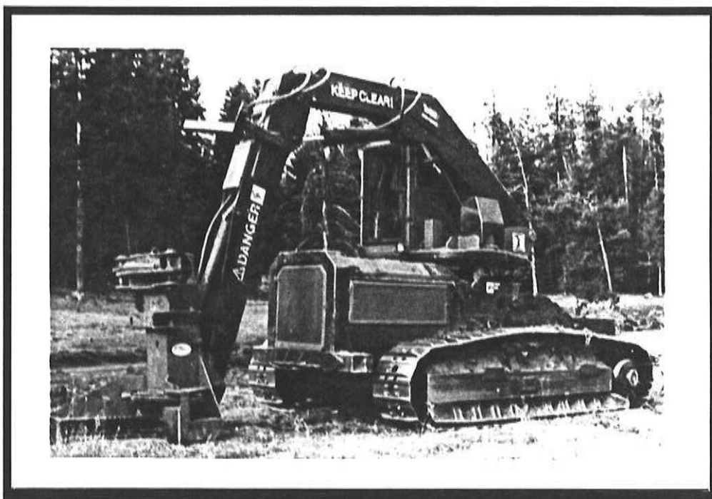
Timbco equipment used in mechanical tree felling, Maloney Creek, 1988. (Photos: T. Roberts, Nez Perce Tribal Forestry Office)
