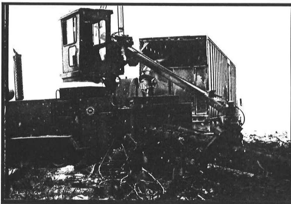
Mechanical precommercial thinning equipment: A Chipper filling trucks on the Mission Creek Reserve, ca. 1982 (above) and on the West Winchester Reserve in 1983 (below). (Photos: T. Roberts, Nez Perce Tribal Forestry Office)
