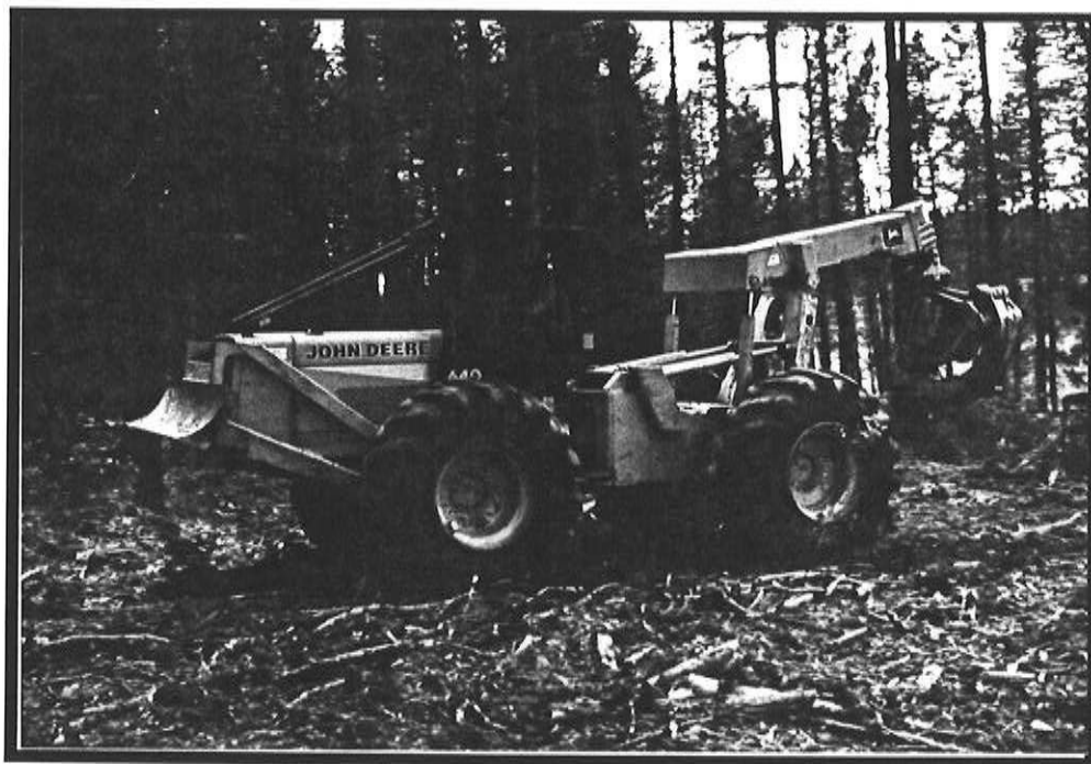
Mechanical precommercial thinning equipment: A rubber-tired Grapple Skidder on the Mud Springs Reserve, T.U. 11, as part of the Hog Fuel Operation, 1982-85. (Photos: T. Roberts, Nez Perce Tribal Forestry Office)
